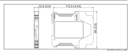
Housing for DIN rail mounting according to IEC 60715; Dimensions in mm (in)
