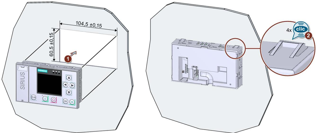
Place the 3RW5 HMI High Feature in the cutout of the control cabinet door ①. Ensure that the 3RW5 HMI High Feature engages audibly in the 4 fixtures ②.
