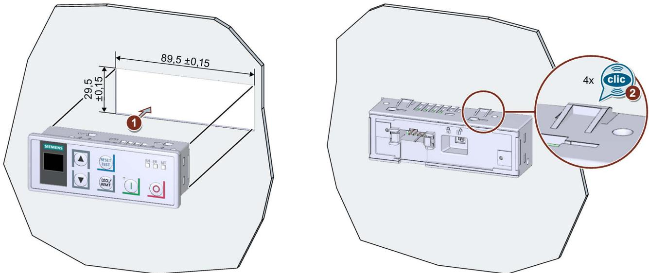
Place the 3RW5 HMI Standard in the cutout of the control cabinet door ①. Ensure that the 3RW5 HMI Standard engages audibly in the 4 fixtures ②.
