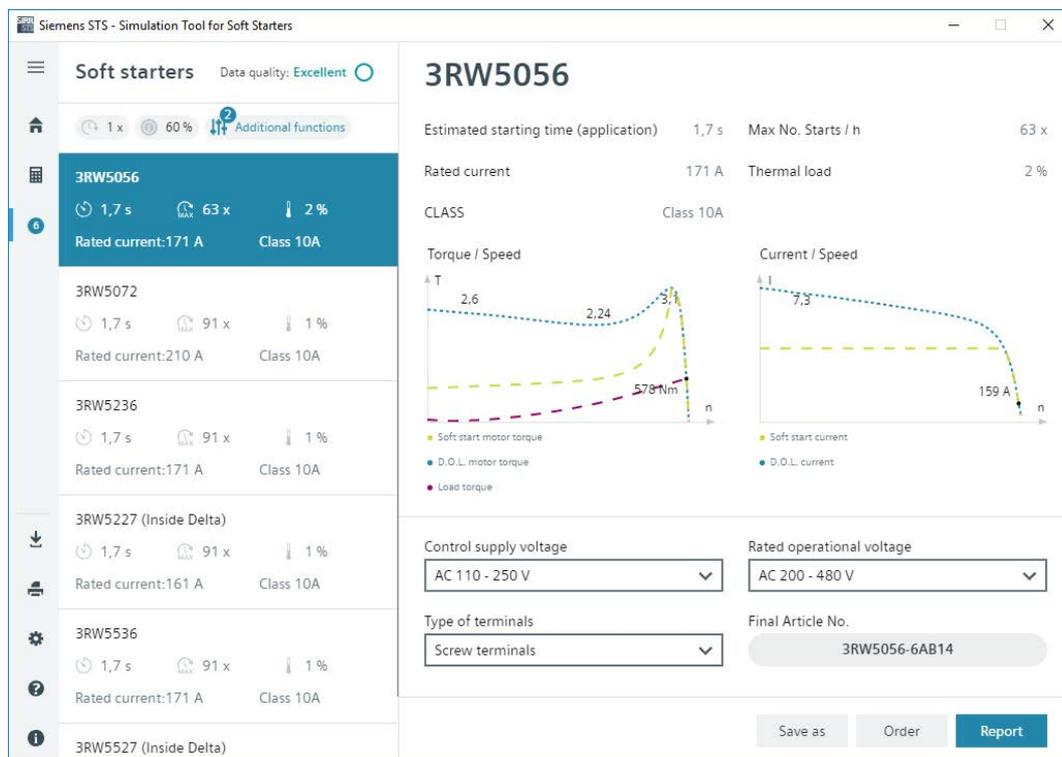
The soft starter can be configured with the STS (Simulation Tool for Soft Starters) software. The STS suggests suitable soft starters for the respective application based on the entered motor and load data and application requirements, as well as providing information on the parameterization.
