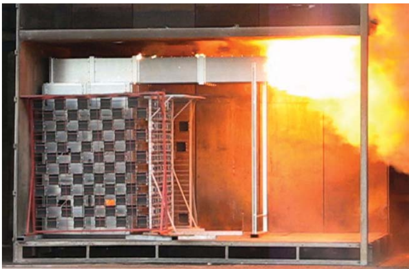
Internal arc fault test, 31.5kA/1s
