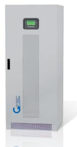
**Libra Pro** is available with a power range from 10 to 100kVA threephase/singlephase and 10 to 800kVA threephase/threephase, using double conversion on-line technology (VFI) with an inverter transformer for output galvanic isolation. The load is powered continuously by the inverter with a filtered, stabilised and regulated sinewave supply. The input and output EMI filters considerably increase the immunity of the load to mains disturbances and surges.
