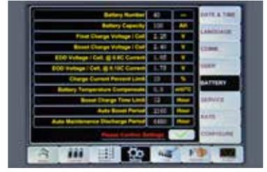
First commissioning can be executed without using any external tools. The three level password protects against accidental accesses and dangerous settings.
