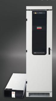
State of the art switch mode technology, N+1 redundant Protect RCS MIPE rectifier system is designed to be scalable, simple to use and easy to maintain with hot swappable rectifier modules. It allows you to benefit from low electromagnetic pollution and high efficiency, resulting in a cost effective system with reduced operating costs, short delivery time and prepared for possible future power expansion.
