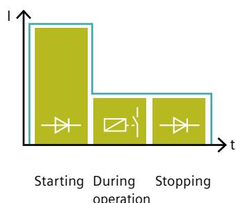
Conventional industrial controls result in wear to the mechanical switching contacts every time a system is switched on or off, albeit in very small increments. This is not the case with hybrid industrial controls, because the starting current is first engaged via electronic contact elements (Thyristor, Triac) and the mechanical contact elements are only engaged when the rated speed is reached. Thus, the mechanical components achieve a significantly higher switching service life.
