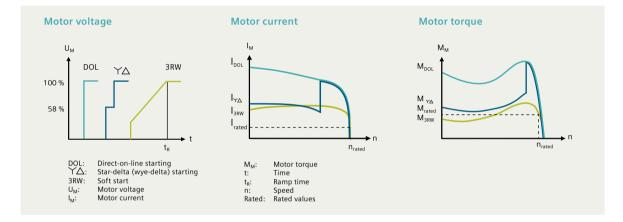
• Considerable savings on wiring in the control panel compared with a contactor assembly for star-delta (wye-delta) starting
