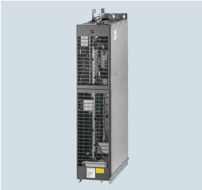
The self-commutated infeed/regenerative feedback units (with IGBTs in infeed and regenerative feedback directions) generate a regulated DC link voltage. This means that the connected Motor Modules are decoupled from the line voltage. Line voltage fluctuations within the permissible supply tolerances have no effect on the motor voltage.
