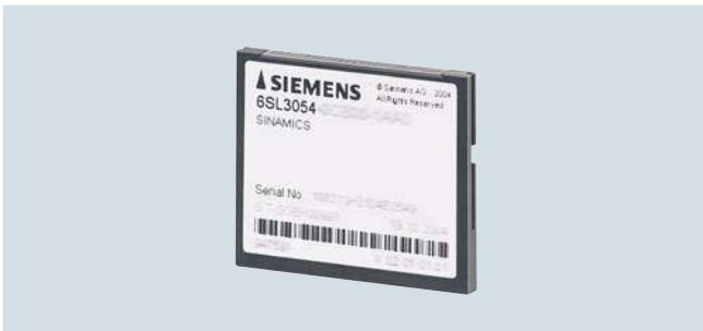
The CompactFlash card contains the firmware and parameter settings. The CompactFlash card is plugged into the appropriate slot on the CU310-2 Control Unit.
