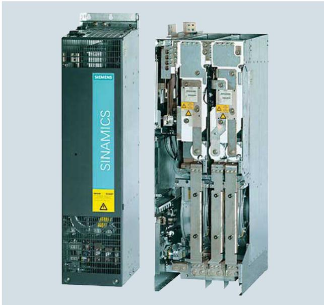
Smart Line Modules are infeed/regenerative feedback units that supply power to connected Motor Modules. Furthermore, they are capable of feeding regenerative energy back into the grid. The in-feed occurs over a diode jumper, while stable, line-commutated regenerative feedback takes place via IGBTs with 100 % continuous energy regeneration. The regenerative capability of the modules can be deactivated by means of parameterization.
