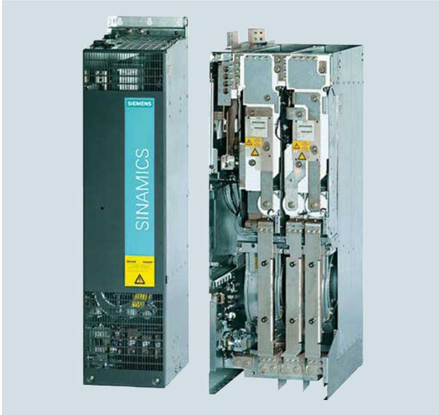
The self-commutated infeed/regenerative feedback units with IGBTs generate a regulated DC link voltage. This means that the connected Motor Modules are decoupled from the line voltage. Line voltage fluctuations within the permissible supply tolerances have no effect on the motor voltage.
