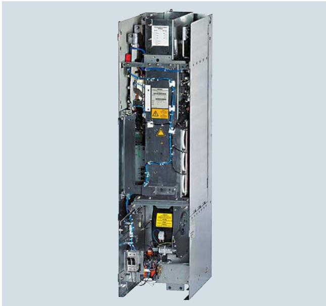
Basic Line Modules are available for applications in which no energy is returned to the supply or where the energy exchange between motor and generator axes takes place in the DC link. Basic Line Modules are designed for connection to grounded TN/TT and non-grounded IT supply systems.
