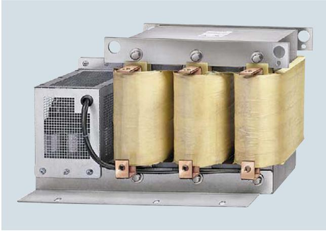
If a sine-wave filter is connected to the output of the Power Module or Motor Module, the voltage between the motor terminals is virtually sinusoidal. This reduces the voltage load on the motor windings and prevents motor noise induced by the pulse frequency.
