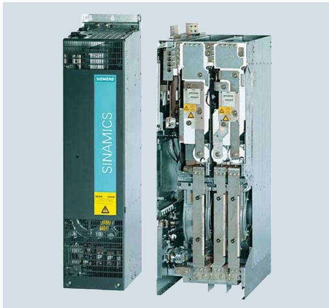
A Motor Module comprises a self-commutated inverter with IGBTs. It generates a variable voltage with variable frequency from the DC link voltage that feeds the connected motor.
