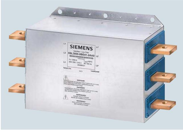
In conjunction with line reactors and a logically consistent configuration of the plant or system, line filters limit the interference conducted by the Basic Line Modules and Power Modules to the limit values of Category C2 acc. to EN 61800-3.
