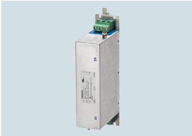
In plants with strict EMC requirements, line filters work together with line reactors to restrict the conducted interference emanating from the power modules to the limit values of Class A1 as defined in EN 55011 and Category C2 as defined in EN 61800-3. Line filters are only suitable for direct connection to TN line systems.
