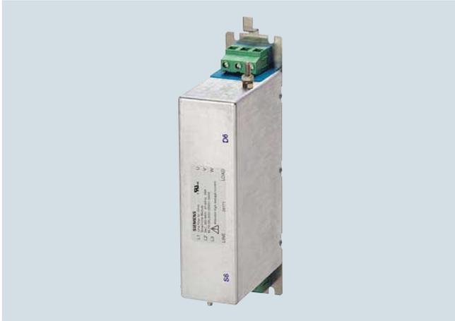
In plants with stringent EMC requirements, line filters work together with line reactors to restrict the conducted interference emanating from the Power Modules to the limit values of Class A1 as defined in EN 55011 and Category C2 as defined in EN 61800-3. Line filters are only suitable for direct connection to TN line systems.
