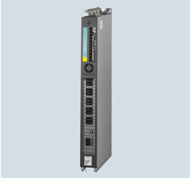
Basic Line Modules are used for applications where energy is not fed back into the line supply or where energy is exchanged in the DC link between axes operating in the motor and generator modes. The connected Motor Modules are pre-charged via the thyristor gate control. Basic Line Modules are designed for connection to grounded TN/TT and non-grounded IT supply systems.
