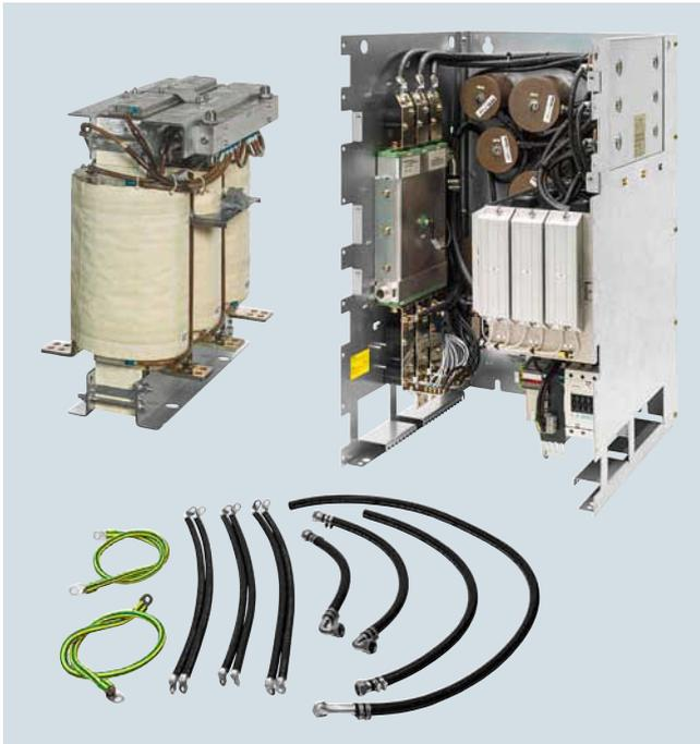
The Active Interface Module essentially comprises a liquid-cooled filter reactor and a liquid-cooled filter module. The filter module contains a Clean Power Filter with basic RI suppression, the pre-charging circuit for the Active Line Module, the line voltage sensing circuit and monitoring sensors.
