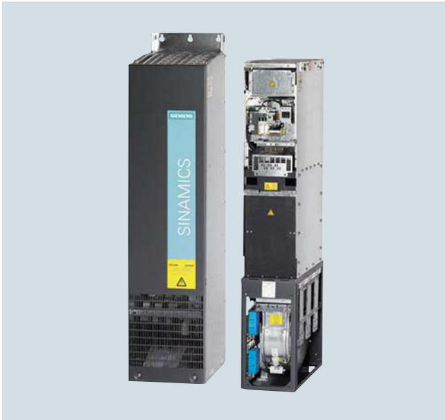
Active Interface Modules are used in conjunction with Active Line Modules. Active Interface Modules contain a Clean Power Filter with basic RI suppression, the pre-charging circuit for the Active Line Module, the line voltage sensing circuit and monitoring sensors. The bypass contactor is an integral component in types FI and GI. This ensures a highly compact design. The bypass contactor must be provided separately for frame sizes HI and JI.
