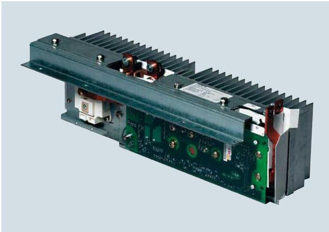
A Braking Module and the matching external braking resistor are required to bring drives to a controlled standstill in the event of a power failure (e.g. with an EMERGENCY STOP) or to limit the DC link voltage for brief periods of regenerative operation, e.g. if the Line Module is not capable of energy recovery.
