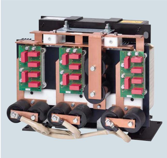
dv/dt filters compact plus VPL (**V**oltage **P**eak **L**imiter) limit the voltage rate-of-rise  $dv/dt$  to values of  $< 1600 \text{ V}/\mu\text{s}$  and the typical voltage peaks to the following values in accordance with the limit value curve A according to IEC 60034-25: 2007:
