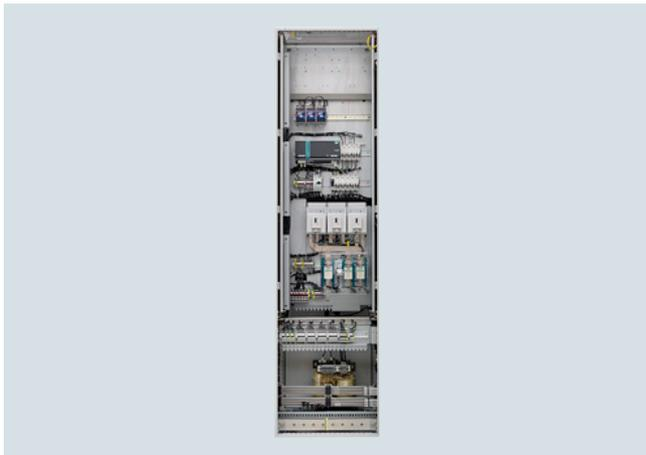
Auxiliary Power Supply Modules supply the auxiliary power supply system for the SINAMICS S120 Cabinet Modules. Units connected to this auxiliary power supply system include the fans of the SINAMICS S120 devices installed in the Cabinet Modules. In addition, the auxiliary power supply system supplies the electronic modules with an external voltage of 24 V DC. This is required when the DC link is not charged, for instance, in order to maintain PROFIBUS/PROFINET communication.
