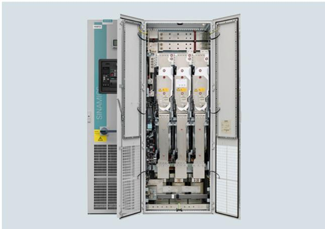
Smart Line Modules are non-regulated infeed/regenerative units. The infeed occurs over a diode jumper, while stable, line-commutated regenerative feedback takes place via IGBTs with 100 % continuous energy regeneration. An autotransformer is not required for regenerative feedback.
