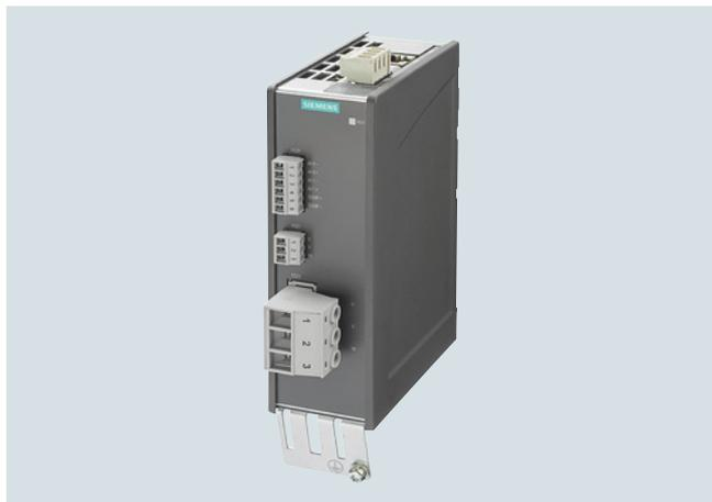
The VSM10 Voltage Sensing Module enables the line or motor voltage characteristic to be measured precisely. The phase differential voltage can be measured, either grounded (in the delivery state with jumper plugged in) or isolated.
