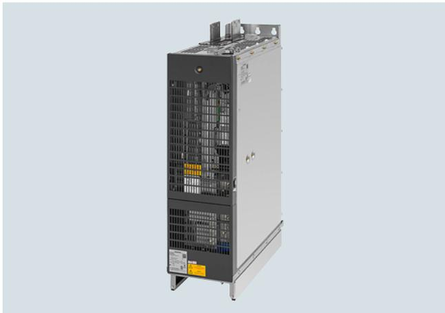
The self-commutated infeed/regenerative feedback units (with IGBTs in infeed and regenerative feedback directions) generate a regulated DC link voltage. This means that the connected Motor Modules are decoupled from the line voltage. Line voltage fluctuations within the permissible supply tolerances have no effect on the motor voltage.
