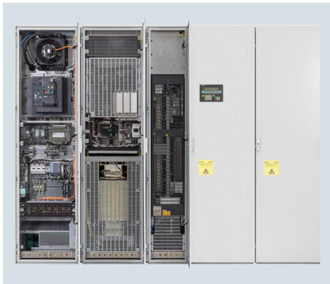
Active Line Connection Modules comprise a Line Connection Module, a liquid-cooled Active Interface Module and a liquid-cooled Active Line Module. They can supply motoring energy to the DC link and return regenerative energy to the line supply.
