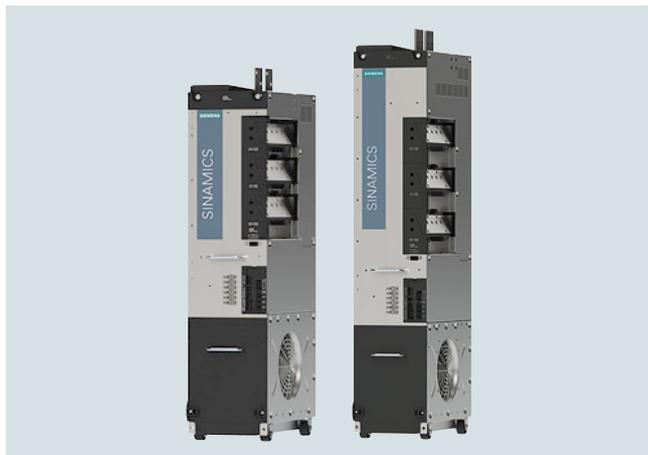
A Motor Module comprises a self-commutated inverter with IGBTs. It generates a variable voltage with variable frequency from the DC link voltage that feeds the connected motor.
