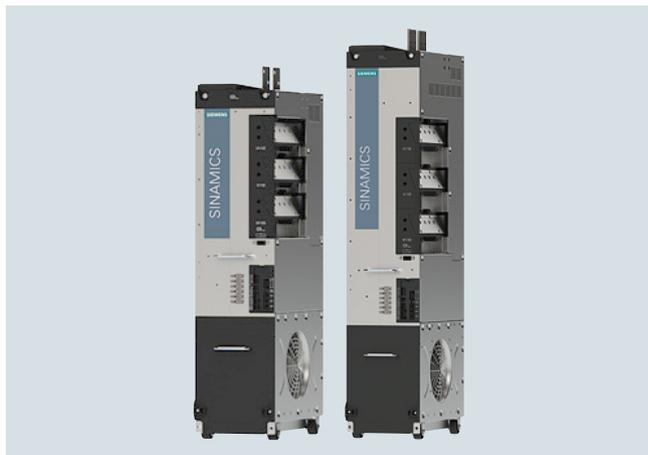
The self-commutated infeed/regenerative feedback units act as step-up converters and generate a stabilized DC link voltage that is 1.5x greater (factory setting) than the nominal voltage of the distribution system. In this way, the connected Motor Modules are decoupled from the line voltage. This improves the dynamic response and control quality because line tolerances and fluctuations do not affect the motor voltage.
