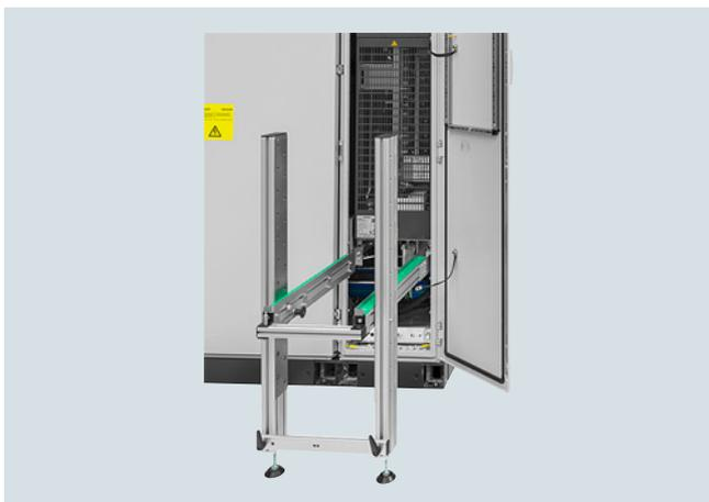
The mounting device is used to install or remove liquid-cooled power units (Line Modules, Motor Modules) in or out of a control cabinet. The mounting device can be used if the power units are mounted on mounting rails, which at the front have two M6 threads at a vertical distance of 20 mm to attach the mounting device.
