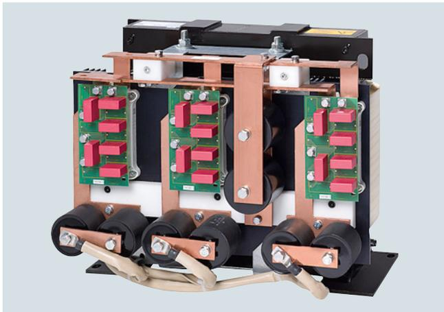
dv/dt filters compact plus VPL (**V**oltage **P**eak **L**imiter) limit the voltage rate-of-rise  $dv/dt$  to values of  $< 1600 \text{ V}/\mu\text{s}$  and the typical voltage peaks to the following values in accordance with the limit value curve A according to IEC 60034-25: 2007:
