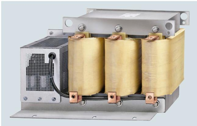
If a sine-wave filter is connected to the output of the Power Module or Motor Module, the voltage between the motor terminals is virtually sinusoidal. This reduces the voltage load on the motor windings and prevents motor noise induced by the pulse frequency.
