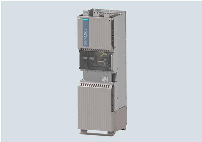
Active Interface Modules in chassis-2 format are used in combination with Active Line Modules in chassis-2 format. The Active Interface Modules in chassis-2 format contain a Clean Power Filter with basic interference suppression, line voltage detection, and monitoring sensors.
