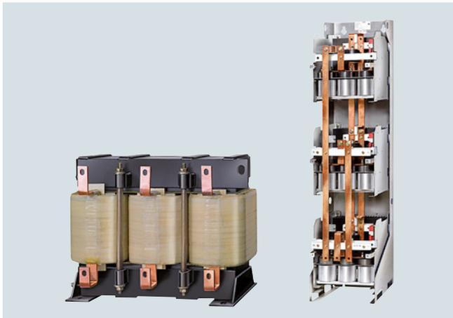
dv/dt filter plus VPL (**V**oltage **P**eak **L**imiter) limit the voltage rate-of-rise  $dv/dt$  to values  $< 500 \text{ V}/\mu\text{s}$  and the typical voltage peaks to the following values in accordance with the limit value curve according to IEC/TS 60034-17: 2006:
