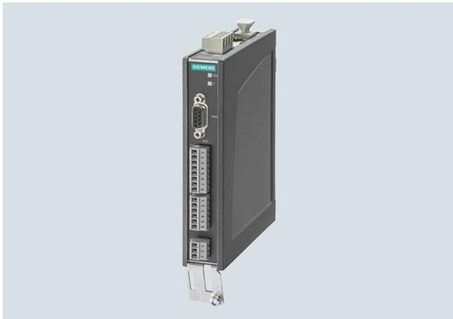
The TM41 Terminal Module supplies TTL signals which emulate an incremental encoder, e.g. to a higher-level control. The encoder interface (incremental encoder emulation) can be linked to an encoder signal from the Control Unit, e.g. incremental encoder sin/cos, by parameter assignment.
