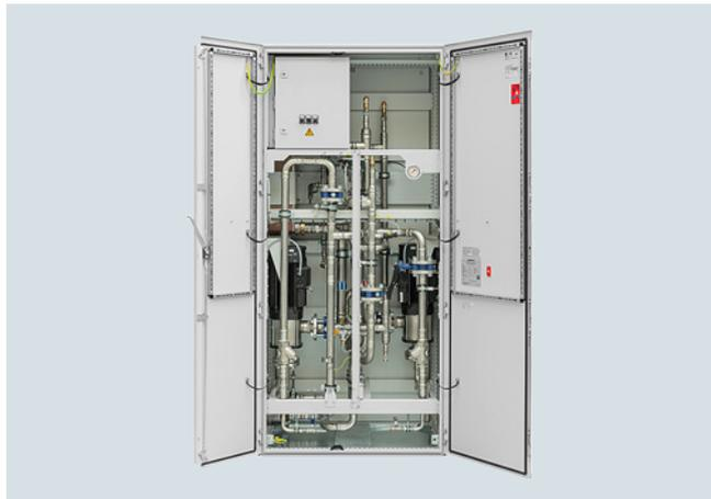
Heat Exchanger Modules are used to dissipate the power loss from the converter. They comprise a deionized water circuit on the converter side and a raw water circuit on the plant side.
