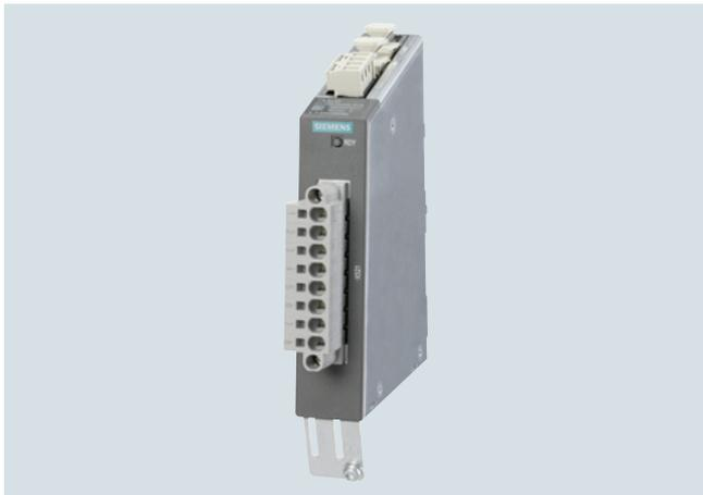
Four temperature sensors can be evaluated via the TM120 Terminal Module. The temperature sensor inputs are safely electrically isolated from the evaluation electronics in the TM120 Terminal Module and are suitable for evaluating the temperature of special motors, e.g. SIMOTICS L-1FN linear motors and SIMOTICS T-1FW6 built-in torque motors.
