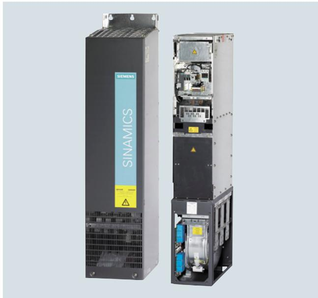
Active Interface Modules are used in conjunction with Active Line Modules. Active Interface Modules contain a Clean Power Filter with basic RI suppression, the pre-charging circuit for the Active Line Module, the line voltage sensing circuit and monitoring sensors. The bypass contactor is an integral component in frame sizes FI and GI. This ensures a highly compact design. The bypass contactor must be provided separately for frame sizes HI and JI.
