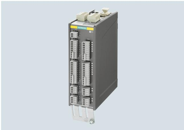
The TM54F Terminal Module is a dual-processor I/O interface with four fail-safe digital outputs and ten fail-safe digital inputs for utilization of the Safety Integrated functions of the SINAMICS drive system via external actuators and sensors.
