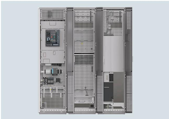
Active Line Connection Modules-2 comprise a Line Connection Module, an Active Interface Module in chassis-2 format and an Active Line Module in chassis-2 format installed in a cabinet system. They can supply motoring energy to the DC link and return regenerative energy to the line supply.
