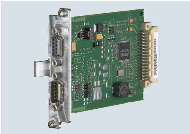
The CBC10 Communication Board is used to interface the CU320-2 Control Unit (and therefore the drive system) to the CAN (Controller Area Network) protocol. The board's driver software fulfils the standards of the following CANopen specification of the CiA organization (CAN in Automation):
